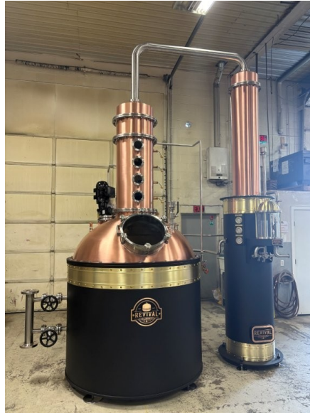
Completed custom copper still at Revival Stillworks. Photo courtesy of Revival Stillworks.
